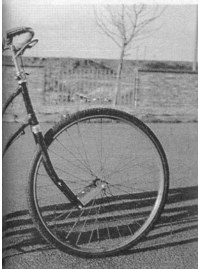
"UNRIDABLE" BICYCLES. David Jones is seen here with three of his experimental machines, two of which turned out to be rideable after all. At top of this page is URB I, with its extra counter-rotating front wheel that tests the gyroscopic theories of bicycle stability. At left is URB III, whose reversed front forks give it great stability when pushed and released riderless. URB IV (immediately above) has its front wheel mounted ahead of the usual position and comes nearest to being "unrideable." —FIG. 1
